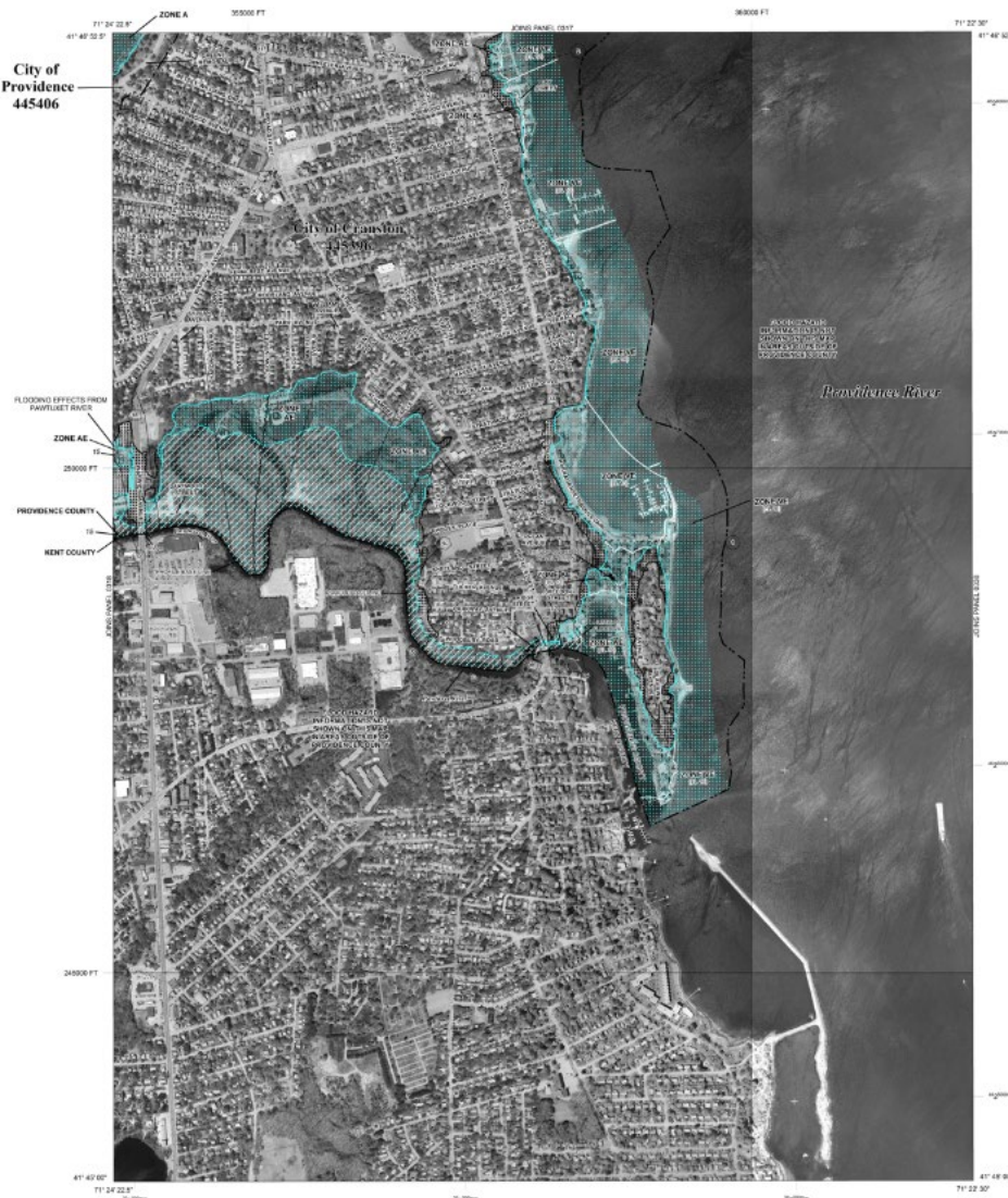
Figure 12-1. FEMA Flood Insurance Rate Map for a portion of Cranston Source: FEMA, 2015
